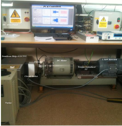
Fig. 2. Test rigs units based dSPACE 1103 hardware
