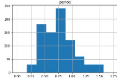
Fig. 2. Distribution of calculated natural periods for the building models
